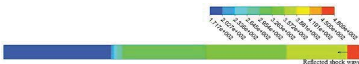
Fig 6. Shock wave reflection from end wall creating high temperature behind shock
